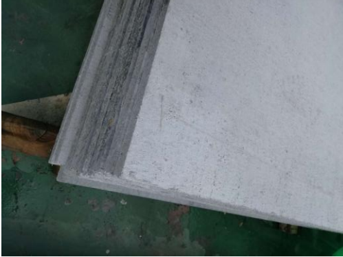
Cement fiber floor
