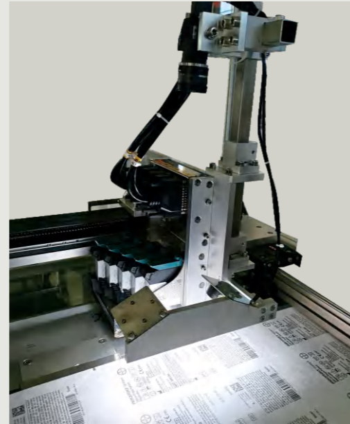
喷码在线视觉检测 In-line Vision Inspection Of Printing
