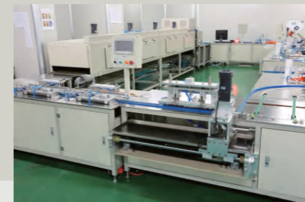
上胶、搓针对向 EPOXY bonding、Cannula adjust
